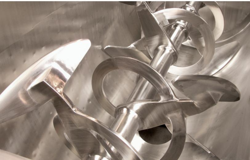
Combining the best of both worlds, American Process Systems® (APS) developed the combination outer paddle and inner ribbon agitator for applications involving fragile and heat sensitive products such as cereals, leafy spice mixes, and to prevent sugars from caramelizing.
