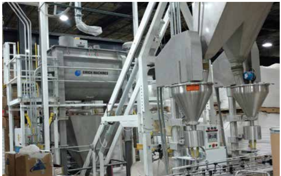
APCO installed an OptimaBlend blender to provide an efficient, high-quality mixture for a new product line.
