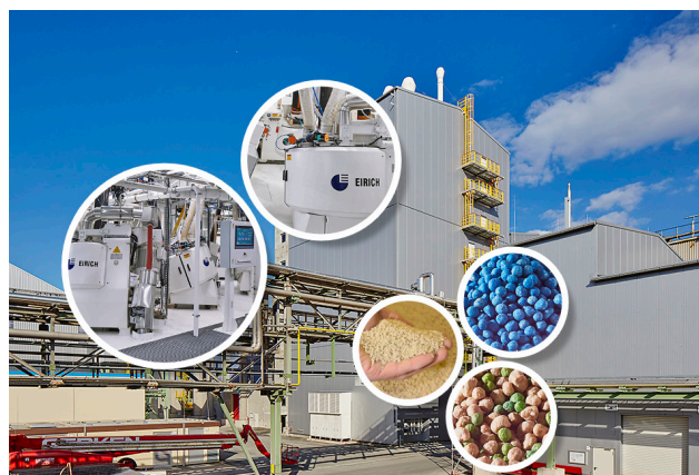
Figure 5. A production plant in Krefeld, Germany, showing the mixing and granulating of NPK fertilizer.
