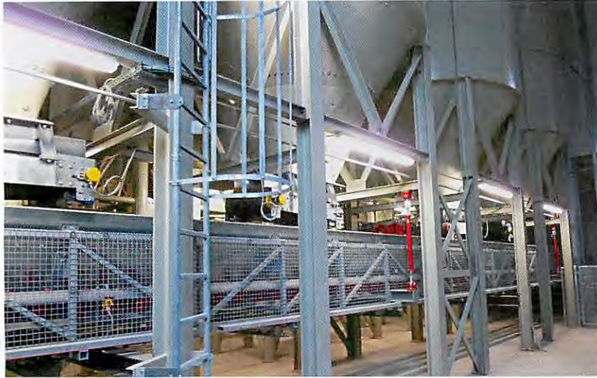
Gasus batching system with weighing conveyor and silos
