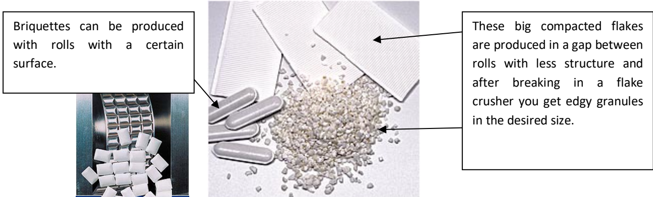
Figure 5: examples for press agglomerates ( www.bepexhosokawa.com )
