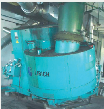
Eirich Mixing Cascade 35 t/h
