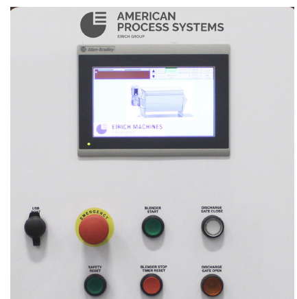
APS performance control panel with 7-inch color screen
