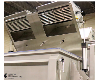
Pneumatically actuated cover
