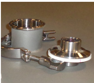
Tri-clamped ferrules for liquid addition port
