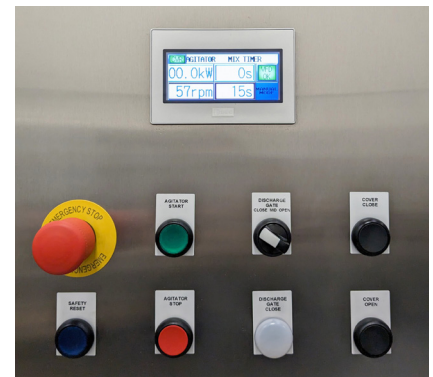
APS standard control panel with 3.8-inch color screen
