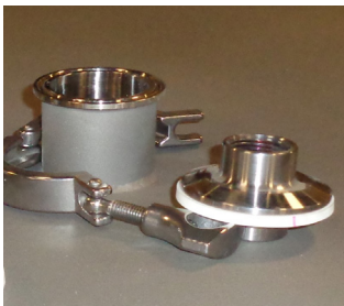
Tri-clamped ferrules for liquid addition port
