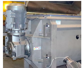
Direct drive, right angle shaft mount
