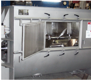
Side access doors
