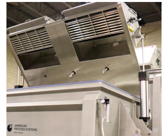
Pneumatically actuated cover
