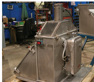
NEMA 9/XP dust electricals
