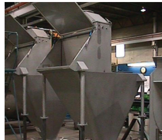
FBD with surge hopper extended to accommodate customer's bulk bag discharge frame
