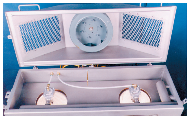
Internally mounted fan, pulse jet cartridge cleaning divertors, and compressed air manifold.
