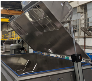
NBD on pneumatically lifted blender cover
