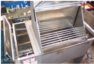
Bag dump on blender with side access covers
