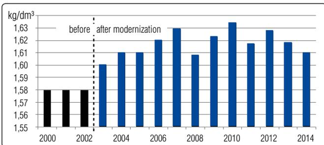
Baked apparent density before/after installation of a remixer-cooler
