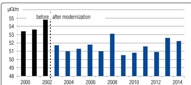
Specific electric resistance before/after installation of a remixer-cooler
