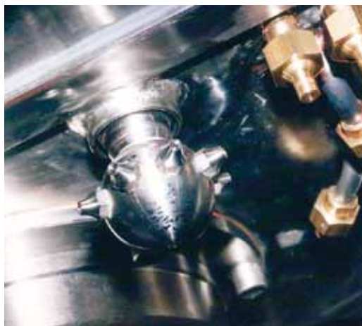
High-pressure cleaning nozzles Pin-type rotor
